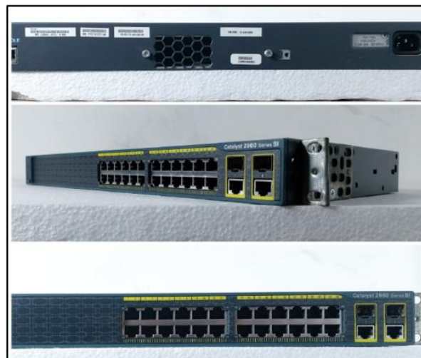
Gbr. 1 Switch Cisco Catalyst 2960
